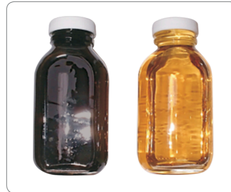
Dirty and clean oil samples, before and after oil filtration. The filter inserts have absorbed the contamination from the crusher oil, and an oil change has now been avoided
