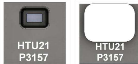
Laser marking on HTU21P(F) sensor
