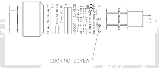
The design features a simple form of adjustment. This enables users to order switches set at a predetermined point or stock a mid range setting and adjust switches to suit the particular application. Rotating the body directly compresses the disc springs, rotation to the right will decrease the set point and conversely moving to the left will increase the set point.
