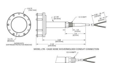
MODEL LTB - GLAND SEAL CONDUIT CONNECTION
