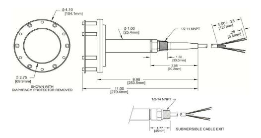
**Molded Cable Seal Configuration for Polyurethane Cable**
