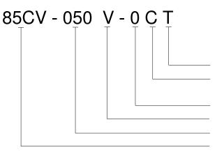
Vent (T = Tube, Blank = No Tube) Electrical (R = Ribbon Cable, C = Cable with Connector) Fitting Type (0 = Weldable, See Fittings) Type (V = Vacuum Gage) Pressure Range Model
