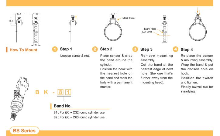
Clamp is designed for mounting KT-48 series sensor on round cylinder.
