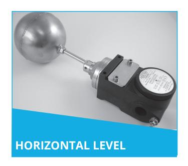
Switching is effected in this unit through transforming, by means of a eccentric cam at fulcrum, the vertical motion of the flow with level change to the considerably reduced movement of a horizontal switch plunger which is arranged to operate a one or two SPDT/SPCO microswitches.
