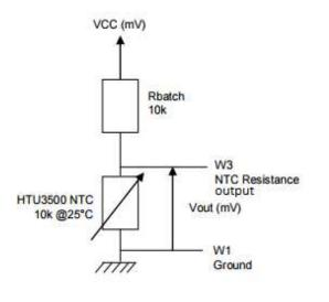
$$V_{OUT}(mV) = \frac{Vcc(mV) * NTC_{HTU3500}(\Omega)}{R_{batch}(\Omega) + NTC_{HTU3500}(\Omega)}$$
