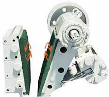
Note: Cupping may occur in the joint of movable jaws if the movable jaw is rotated when it is installed in the lower position. This may decrease the crusher's capacity and increase wearing on the fixed side.
