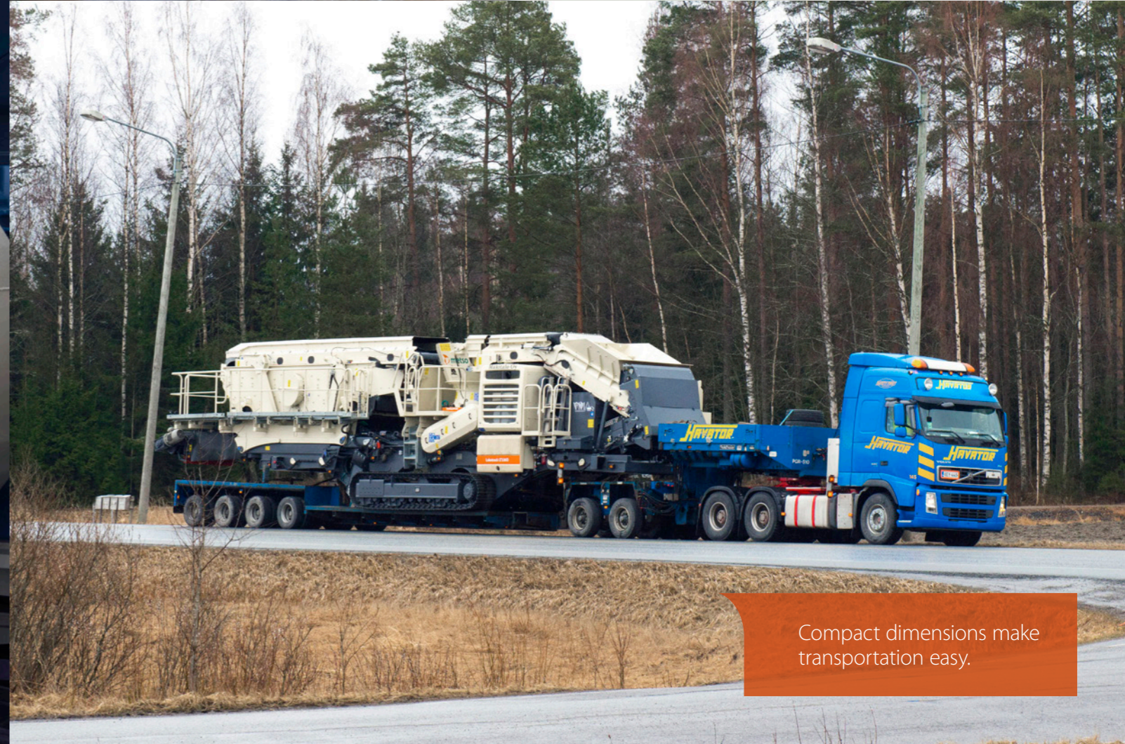
At 2 000 mm (6' 7") wide, the dual-slope screen has been purposely designed for heavy-duty screening.
