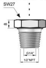
N2 type 1/2"NPT male + internal thread G1/4"
