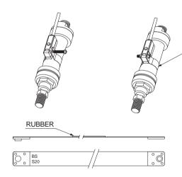
Wrap the band around cylinder barrel and re-insert screw head into clamp. Position the switch and tighten.
