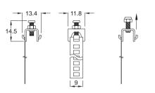
Step 1 Loosen screw & nut.
