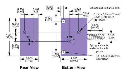
Two through holes and four 3 mm x 0.5 mm threaded holes are provided for mounting
